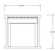
Grates longer than 1500mm supplied in sections. Tile Inserts longer than 1200mm supplied in sections. Channels over 3000mm supplied in sections with joiner. +/-2mm tolerance on dimensions.
