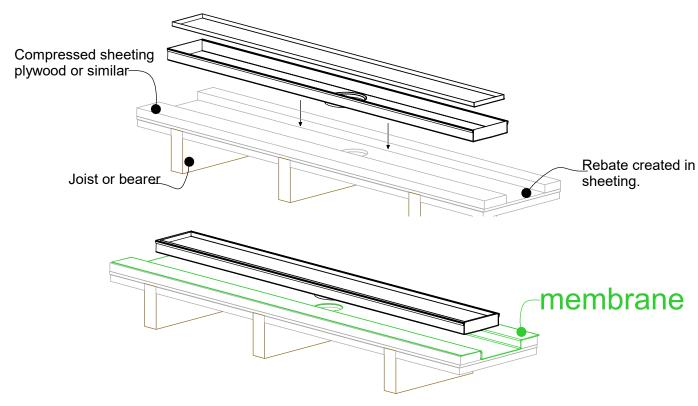
NOTE: For exterior application allow for expansion of 1mm per 3 metres by using quality suitable flexible sealant on channel joins.
